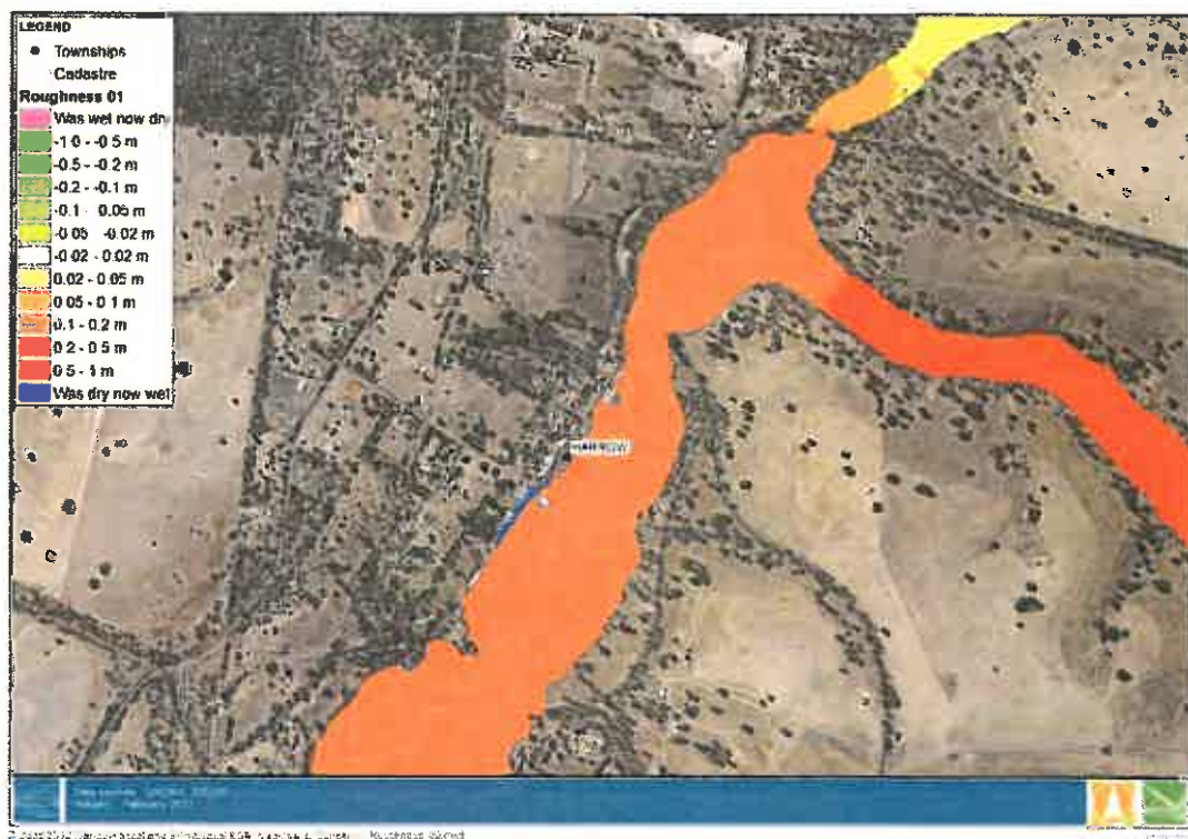
Figure 7-6 Change in water levels and extents due to a 10% increase to all roughness values
