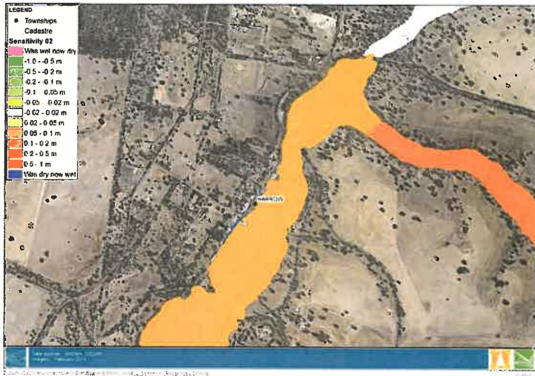
Figure 7-3 Difference in water level due to the 14.5 m 3 /s Rocklands release - Depths at Harrow
