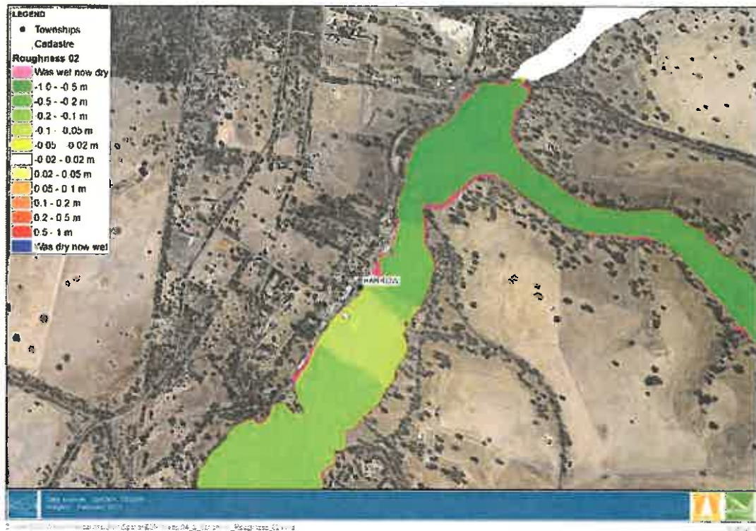
Figure 7-5 Change in water levels and extents due to an unrealistically decreased floodplain roughness
