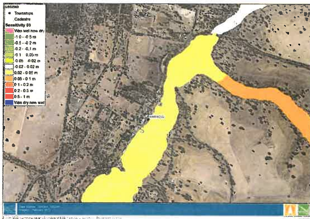
Figure 7-4 Difference in water level due to the 6.9 m 3 /s Rocklands release - Depths at Harrow
