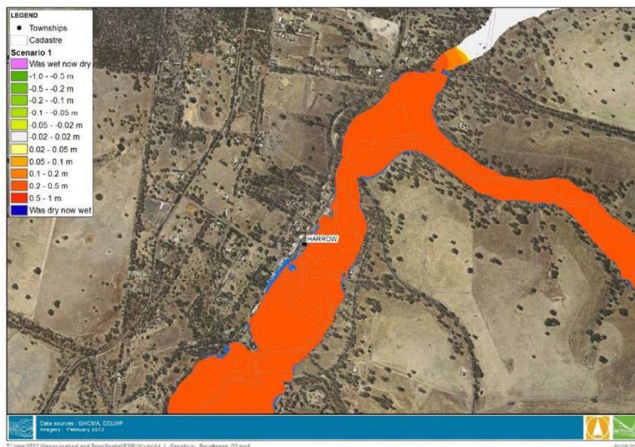
Figure 7-2 Difference in water level due to the 61.3 m 3 /s Rocklands release depths at Harrow
