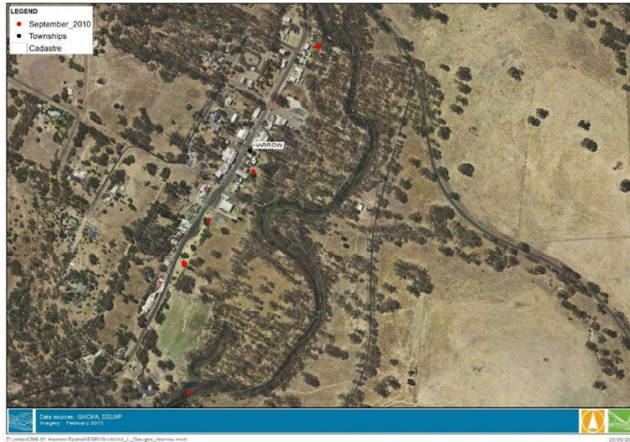
Figure 6-8 Location of September 2010 surveyed flood marks
