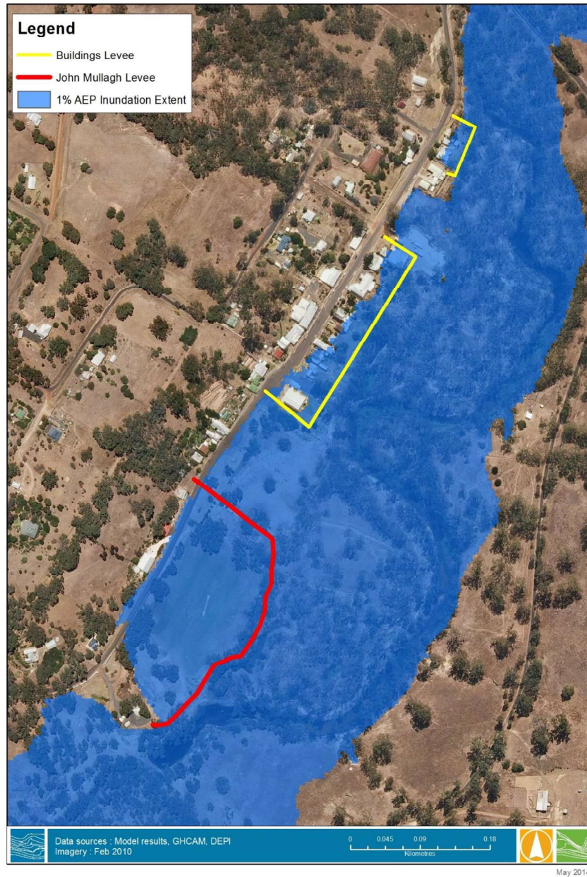
Figure 8-4 Assessed levee alignments in Harrow
