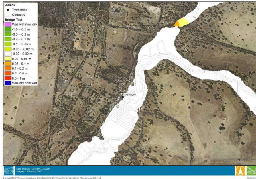
Figure 7-7 Change in water level due to a 10% blockage of the Coleraine Edenhope Road
