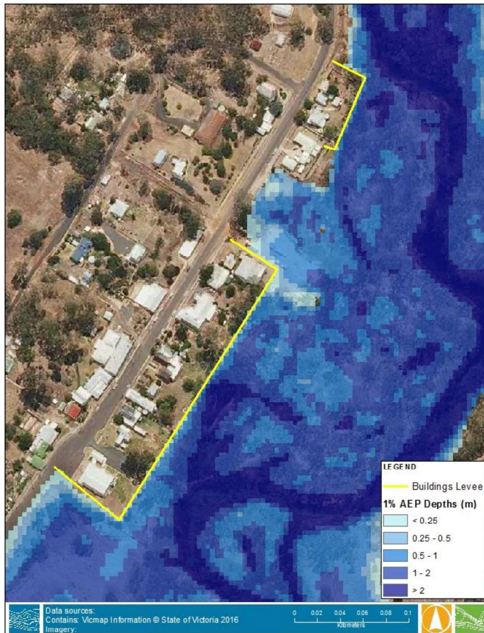
Figure 8-5 Buildings Levee Alignment and 1% AEP depths
