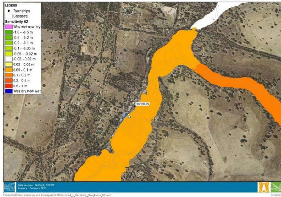
Figure 7-3 Difference in water level due to the 14.5 m³/s Rocklands release - Depths at Harrow
