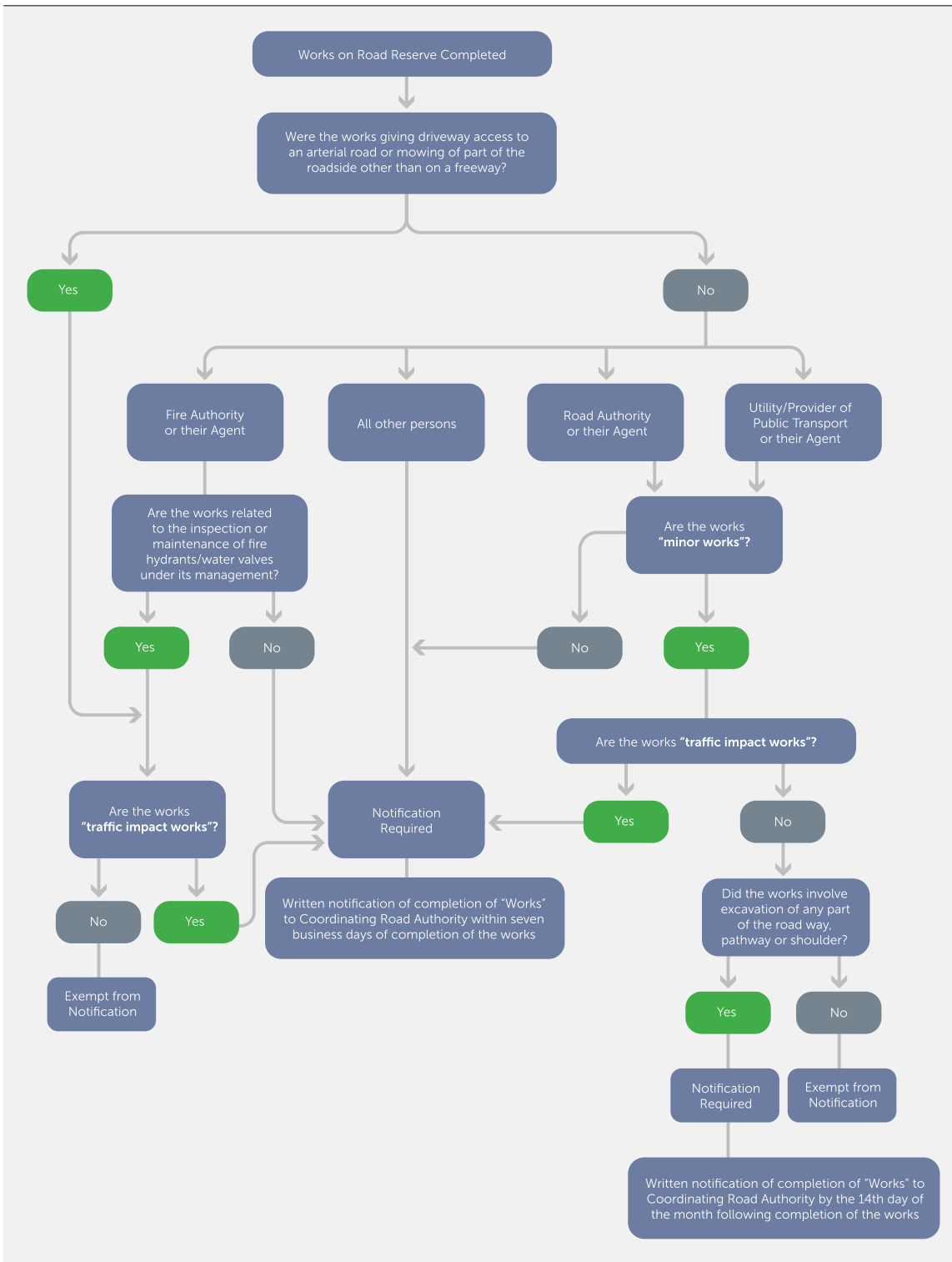
Flow Chart 3 Notification of Works Completion to Coordinating Road Authority by Works Manager
